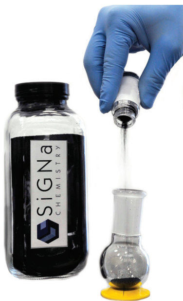
Stage I Na-SG being poured through ordinary laboratory air
